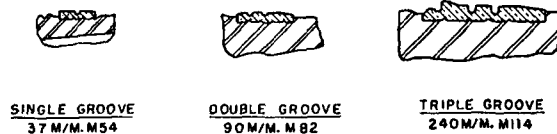
TYPES OF ROTATING BANDS FOR ARTILLERY PROJECTILES
